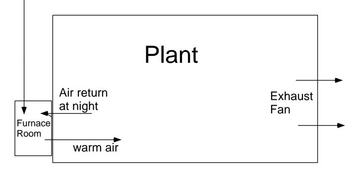
At night, when exhaust fans are off, the vent to the outside is shut and a return vent from the plant is opened so warm air from the plant can be circulated through the furnace room
